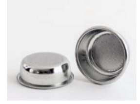
The filter shape with a rounded internal corner concentrates extraction towards the centre of the coffee puck, avoiding those sections where the ground coffee is not well exploited during the extraction process. This is combined with an M type of perforation that has a greater concentration of holes in a restricted area.
